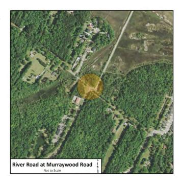
and the entire Murraywood Road to a four-lane facility will be required to accommodate the future traffic projections. The proposed geometric modification will improve the afternoon peak hour operating condition to LOS C (delay 21.6 sec/veh).
