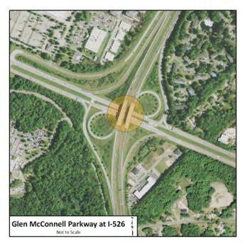
timing improvements. The Glenn McConnell Parkway at Frontage Road intersection will be fully closed due to safety constraint created by the upstream interchange merge/weave conflicts. An at-grade centralized signalized SPUI will be constructed for the Glenn McConnell Parkway and I-526 interchange and additional through lanes will be added to Glenn McConnell Parkway.
